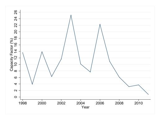
Figure 1.3: Capacity Factor for Steam Condensing Generators, 1998-2011
