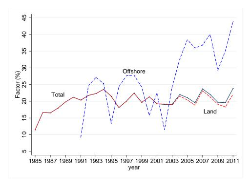
Figure 1.4: Capacity Factors, Wind Turbines, 1985-2011
